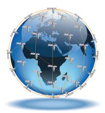
An Iridium Pilot voice or data call is received by the closest satellite to the device's current location, anywhere on the Globe. The traffic is routed through the meshed satellite network and lands at the Alaska Ground Station, and, is then routed over terrestrial networks to the Gateway in Arizona. At the gateway, traffic is converted back to internet protocol (IP) and voice, depending on call type and delivered to the IP cloud or the public switched telephone network (PSTN).
