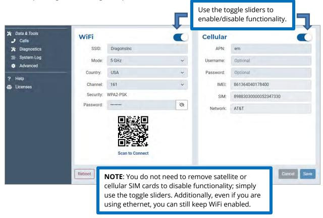
The WiFi section allows you to edit the SSID, Mode, Channel, and randomly generated Password fields. It also contains a scannable QR code for automatic connectivity. When set to 2.4GHz, the Mode field will default to the radio channel with the strongest WiFi signal, and you can select among 11 channels. Changing it to 5GHz will provide you with a new set of channels to choose from.
